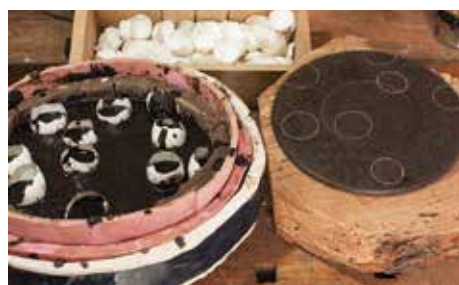
Eggshells cast in a mixture of recycled coffee grounds and epoxy resin (left) and a turned plate revealing the cross-section of eggshells (right).
